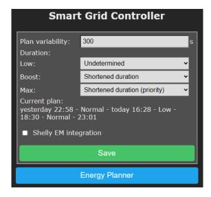
**Plan variability:** On default, the time variation of the plan is 300 seconds (5 minutes). This means that the start time variation will be 300 seconds or less, and the stop time variation will be 300 seconds or less. Random numbers between 0 and 300 seconds will be used to adjust the start
