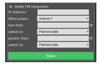
**Shelly EM integration:** With a Shelly EM it is possible to measure the electrical power on a wire.
