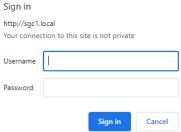
The Smart Grid Controller (SGC) is accessible via the assigned IP address or - if your phone supports mDNS – via the hostname of the switch (e.g. http://sqc.local). The IP address may change if your WiFi network assigns another IP address to the SGC, for example when the SGC has been disconnected from the outlet for some time, and reboots. The hostname however will remain the same, and might be more convenient to use.
